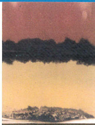
F2. - Diesel Tank Bottom Sample w Microbes
